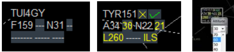
Figure 2 - Controller display for interaction with speech recognizer. Left: 5 interactive cells without contents; middle: speech recognizer output in yellow; right: drop down menu
