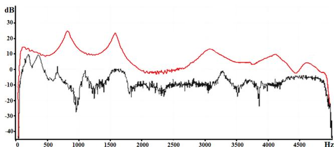
**Figure 2** Measured transfer function of vowel [a:] before (black) and after (red) using a wooden board and clay around the loudspeaker to reduce the cross-talk in the experimental setup. Also, better articulation of vowels and the use of a pulse train led to improved transfer functions. The difference in intensities was a result of the variation of the microphone sensitivity. The measurements were made with the in-house software "Measure Transfer Function".
