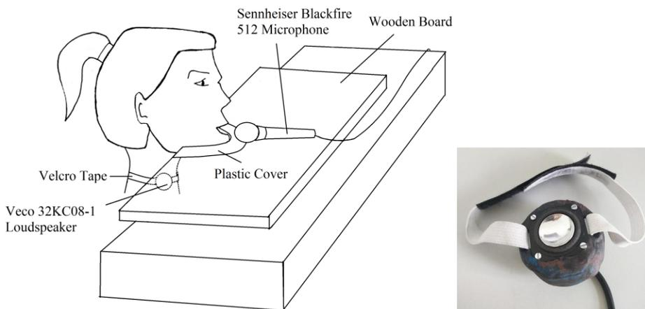
**Figure 1** (Left) The proposed experimental setup. The loudspeaker excites the vocal tract near the subject's larynx with an exponential sweep signal. The wooden board is placed firmly on a desk acting as an acoustic barrier to minimize the cross-talk. The subject sustains articulation of a vowel for the duration of the signal. (Right) Magnified view of the loudspeaker in a box acoustically sealed with clay.
